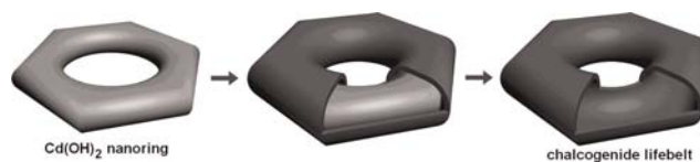
Fig. 1 Scheme of fabrication of the lifelbels by a sacrificial template method.
